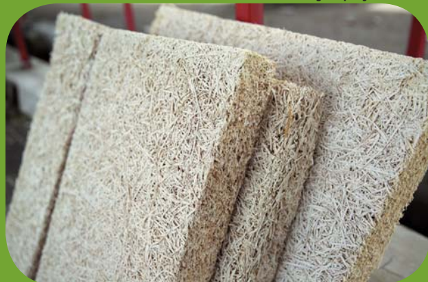
Wood wool cement panels used to build the walls of the home.
